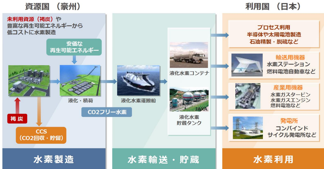
Figure 8 Concept of CO 2 -free hydrogen supply chain 8
